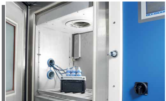
Long-term test at -40 °C in the climatic chamber
