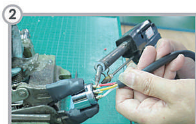
使用夾具將接頭夾持住，線材裸線與上固定體的接觸體缺口進行焊線加工 Using the clamp to fix the connector Doing soldering assembly between the bar wire and upper body
